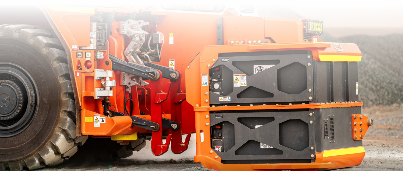
Battery Electric Truck Swapping A Battery At AngloGold Ashanti's Sunrise Dam Operation
