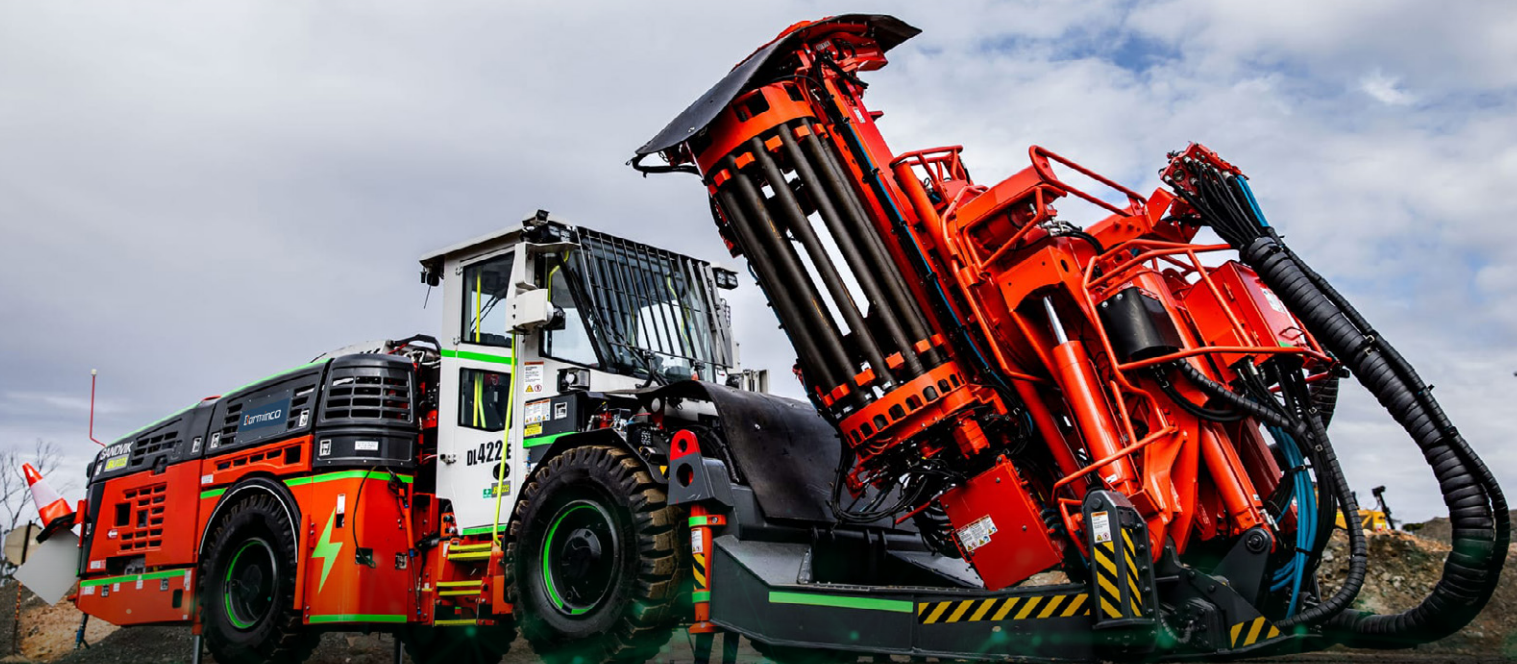
BEV Longhole Drill At The IGO Nova Operation
